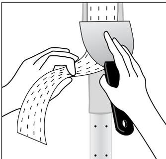
Center a strip of wallboard tape over the joint, and press it firmly into the wet bedding compound with your wallboard knife at a 45° angle. Press hard enough to squeeze a little compound out from the edge of the tape, but leave enough compound for a good bond. Let dry about 24 hours.
