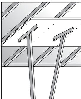
Fireguard X™ gypsum board or  $\frac{1}{2}$ " (12.7 mm) ToughRock® Span 24® ceiling board.
