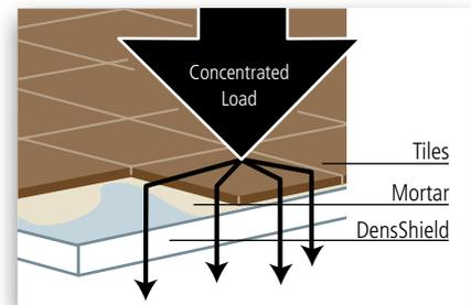
The drawing above depicts how a load is distributed over the surface of a tile and carried by DensShield Tile Backer. With a minimum tile size of 2" x 2" (51 mm x 51 mm) a load of over 1800 lbs. (816 kg) is needed to overcome the compressive strength of DensShield and floor assembly.
