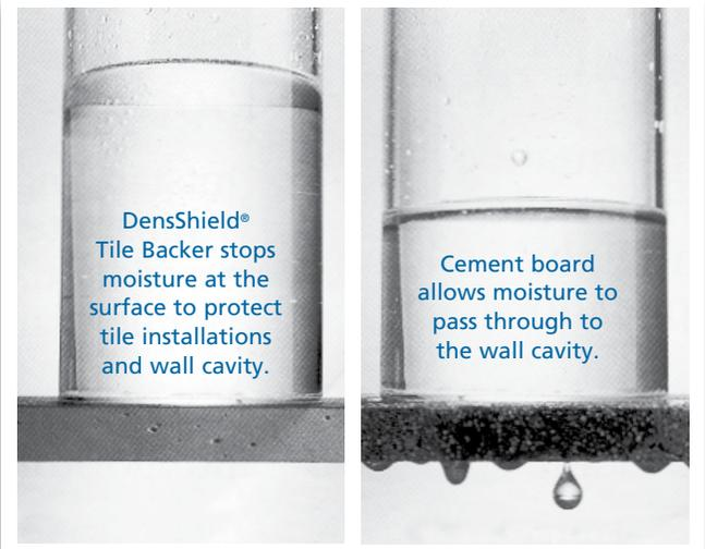
**The test demonstrates DensShield Tile Backer stops water at the surface, while cement boards allow water to pass through their porous construction.** The Tile Council of North America requires the use of a membrane in wet areas for cement backer boards but does not require a membrane for DensShield Tile Backer since DensShield Tile Backer panels have a built-in moisture barrier that stops moisture at the surface.
