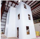
Trial 2: Fluid-Applied Membrane WRB-AB System
