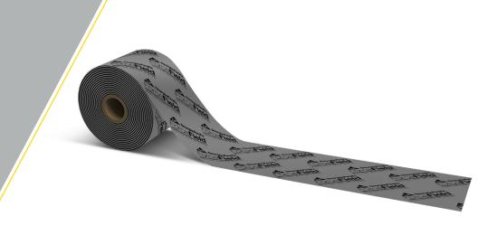
**ForceField® Seam Tape** is a pressure-sensitive polymeric film with an acrylic adhesive used to treat panel seams in the ForceField Weather Barrier System. The ForceField Seam Tape tears easily for a quicker install and is ideal for residential construction projects.
